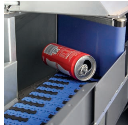
The crate separator actively deflects the empties
