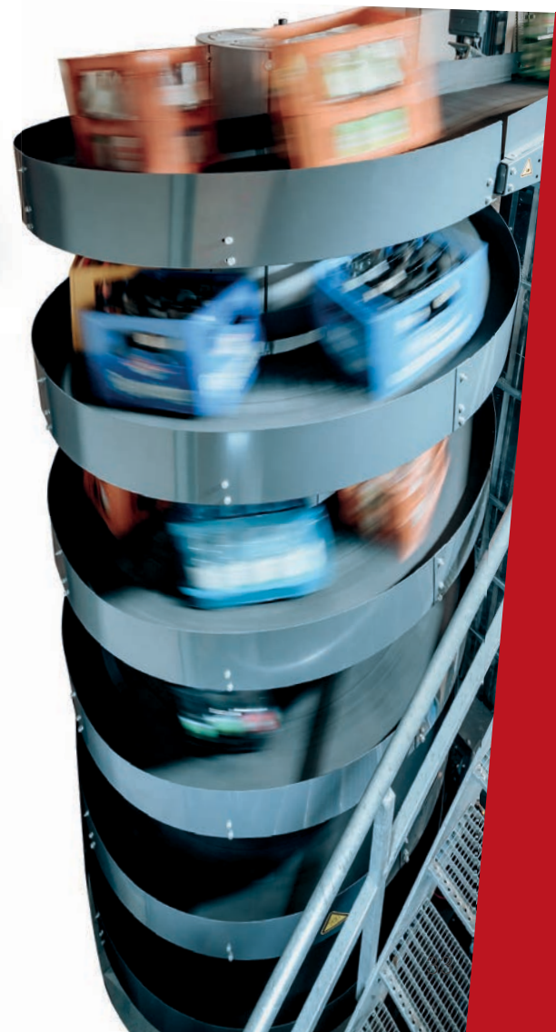
Helix conveyor for transportation with large height differences
