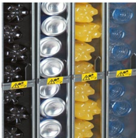
Narrow and standard chutes are combined to offer the best product diversity
