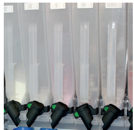
„SiTwist'n Lock“: Instant product container lock with a visual indicator for open (green) and closed (red)
