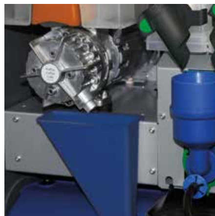
Direct transfer of fresh ground product from the grinder into the brewer via a funnel.
